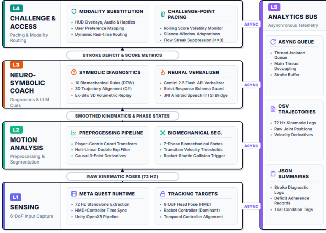
Figure 2: Five-layer system architecture. Sensing data flows upward through Motion Analysis, the Neuro-Symbolic Coach, and the Challenge & Access layer, with an Analytics bus recording telemetry asynchronously at 72 Hz.
